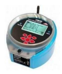
95. The instrument contains three highly sensitive piezoelectric systems for vibration measurement of all three special dimensions. The signal processing is controlled by a microprocessor. The VM40 is operated via its seven keypad buttons and illuminated LCD display. The measurement data can be transferred to a PC via the USB interface. The instrument also has a port for connecting a charger and a relay output for the external signaling of vibration occurrences.
