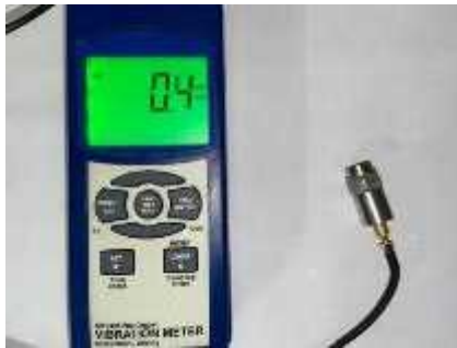
Figure 3: REED instruments SD-8205 model adapter
